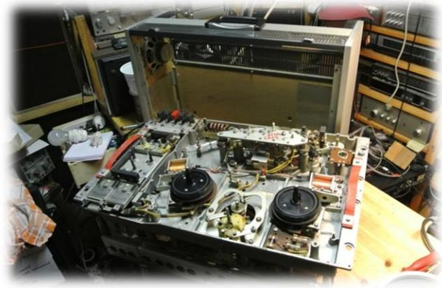
What also stands out are the winding motors, big alternating current types. I have never seen these in consumer recorders from Philips. They also ensure some extra weight. The capstan motor looks familiar and resembles the capstan motor of the Philips consumer recorders such as the N4407.
