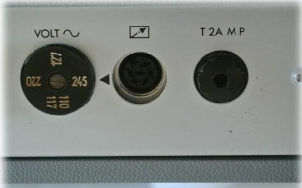
At first I changed the power carousel to 245(V). The average voltage of the contemporary electricity connections of our homes is about 230(V) nowadays. The setting of the power carousel on 220(V) is too low, it could damage the old electronic components.
